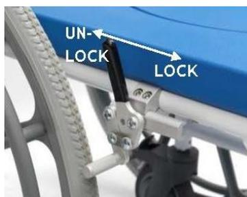
Push the brakes forward to lock the wheel. Pull the brakes back to release the brake. Ensure both brakes are applied when the chair is stationary and when the user is side transferring.
