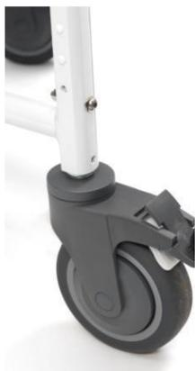
The height of the chair and seat can be altered by adjusting the castor height. To adjust the castor height, remove the 'E' clip or nut and bolt (arrowed). Reposition the castor stem to the required position and reattach the 'E' clip or nut and bolt. Repeat for the 3 castors ensuring they are all set at the same height.
