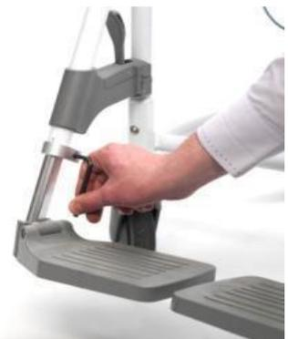
2. To adjust the footplate angle, slacken the bolt near the bottom of the inner tube (chrome). Adjust the footplate to the required angle and resecure the bolt.
